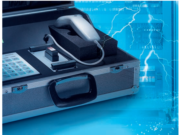
Fig. 7.2-1: Arrester testing device CHECKMASTER
